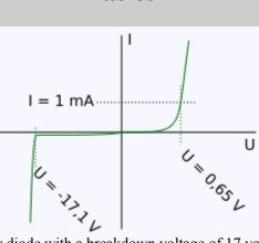
Current-voltage characteristic of a Zener diode with a breakdown voltage of 17 volt. Notice the change of voltage scale between the forward biased (positive) direction and the reverse biased (negative) direction.
